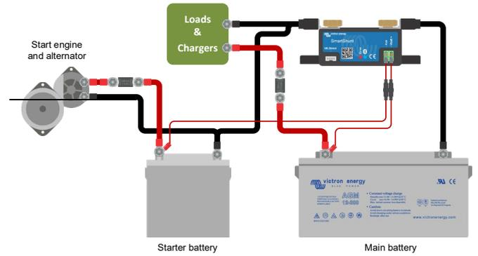
Measuring voltage of the starter battery
